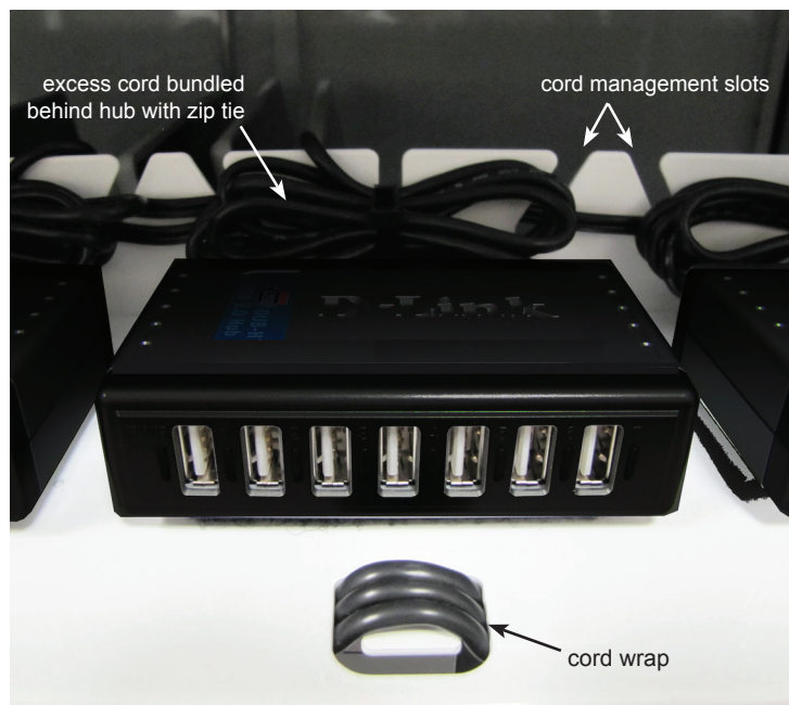
Typical Wiring Recommendation
