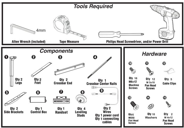
Please count all pieces before disposing of any carton or packing material. Use a padded or carpeted area for assembly to avoid damage. For ease and safety, we recommend two people for assembly.
