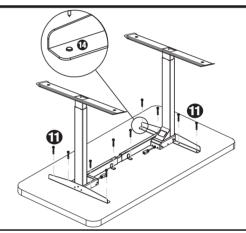
IN THIS FOLLOWING STEP, DO NOT OVERTIGHTEN SCREWS. OVER TIGHTENING COULD J. CAUSE THE PLASTIC ON THE COMPONENTS TO BREAK.
