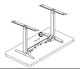
Double-check that the base is centered on the underside of the desktop and is located where Ι. you want it. Also, double-check that the included wood screws are not too long for your desktop and won't puncture the surface when screwed all the way in.
