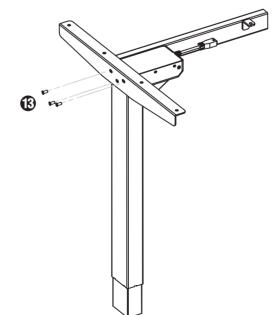
D. Once all of these screws have been started, you can now tighten the gty 4 Flat Head Screws (Part #14) from Step C and the gty 8 Machine Screws (Part #10) described in Step B (12 screws in total).
