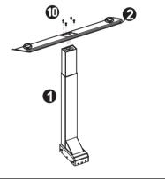
Secure the Center Rails at both ends Η. using qty 4 Machine Screw (Part #10), qty 4 per side.
