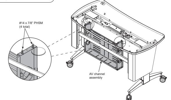
Note: Mounting slots in the undermount AV channel are designed to provide multiple mounting options for AV over IP decoders or other light AV electronics.
